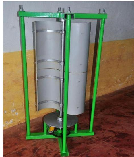
Fig 3(a): Schematic of assembly (b) Photograph of Fabricated model of single stage two blades Savonius wind turbine
