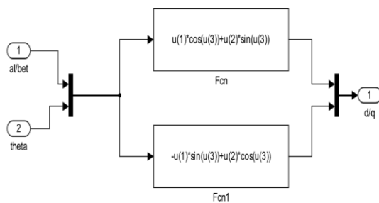
Fig 2.3: Simulation Model of Clarke's to dq transformation
