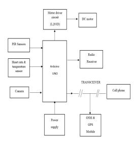
Here above represents the block diagram of live human detection robot
