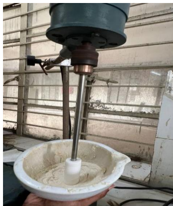
FIGURE LIX HIGH SPEED HOMOGENIZER TO COVERT INTO MICRO-FORMULATION
