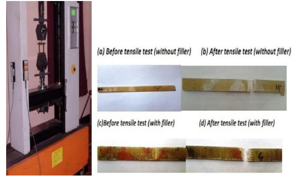
Fig. 3.3 specimens and experimental set up for tensile test.
