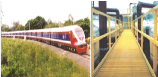
(g) train made up of frp composites (h) composite hand rails and grid
