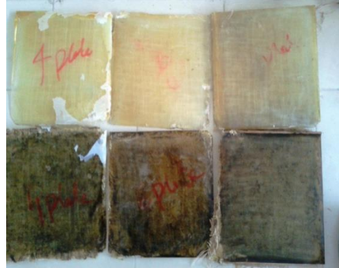
Fig. 3.2 different samples of glass fiber reinforced polymer composites with & without filler (mustard cake powder) fabricated by hand- lay- up techniques.
