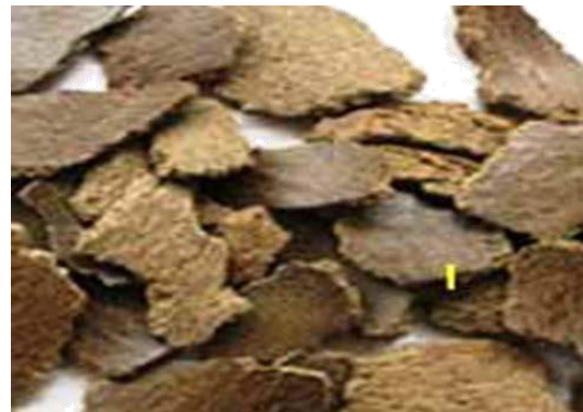
Fig. 3.1 raw materials of filler (mustard cake) used in fiber glass reinforced
