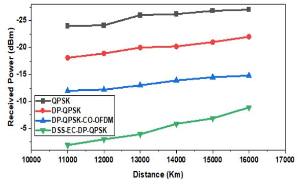
Figure 6 Received Power versus IsOWC distance for diverse modulations
