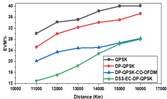
Figure 5 Performance of different modulations at varied IsOWC distance in terms of EVM%
