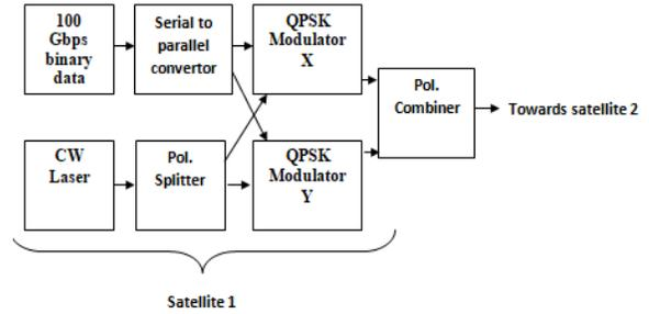
Figure 2 (b) Representation of internal structure of DP-QPSK and Transmissions channel
