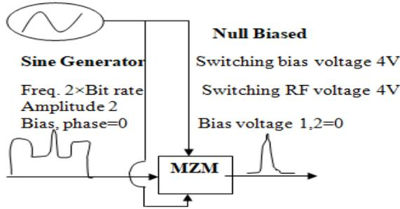
Figure 1 Generation of DSS carrier
