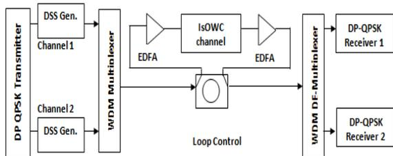
Figure 2 (a) Proposed 100 Gbps/λ WDM-IsOWC system using DSS-DP-QPSK
