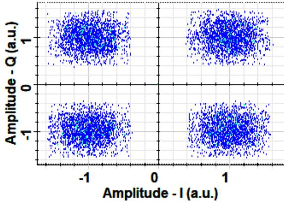
Figure 7 Constellation diagram of proposed DSS-DP-QPSK system at 16000 km IsOWC distance
