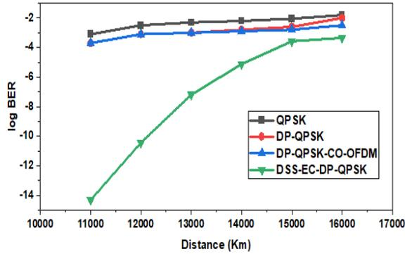
Figure 4 Effect of IsOWC distances on log BER for different modulations
