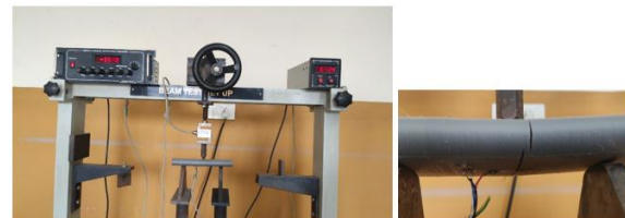
Figure. 1(a) The experimental set-up used for the testing of honeycomb-structured 3D printed sandwich panel
