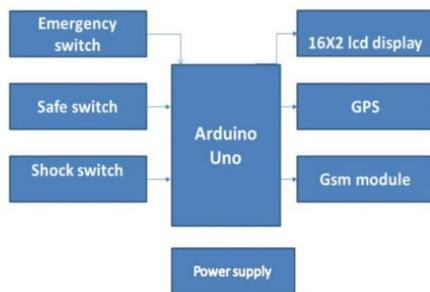
FIG:9 Block diagram of our proposed system
