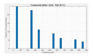
From above figure we can see that total contribution of harmonic component t is about 29.11% when non-linear load is producing harmonics in utility grid.
