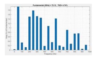
Below is the result when APF is switched on after 0.5 sec and via circuit breaker the reactive power compensation is being performed by harmonic current injected by active power filter. The total harmonic distortion is coming down to 4.74% which is acceptable limit as per IEEE guidelines.
