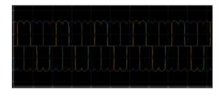
After switching the APF operation the harmonic current is injected into line and this mitigates the harmonics component of current. The Hysteresis current control generates the pulse using below references from source side to drive six IGBT switches of inverter of shunt APF.
