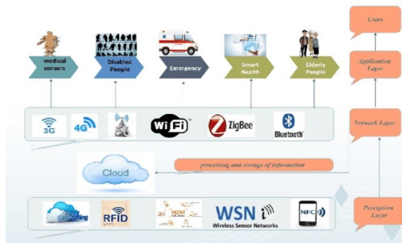
Fig 3: Architecture of Healthcare system in IoT [15] Now we are going to discuss the three layer architecture of IoT technology in healthcare system. It has three layers, to be specific, the perception, network, and application layers.
