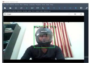
When the person is not wearing helmet the system searches for the number plate in the frame. Once detected it extracts characters and prints on the console.
