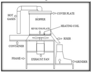
This setup induces hot air into the system with the help of blower. In the furnace, drying process of pulp takes place. Blower increases the rate of heat transfer which in turn decreases the time of reducing the moisture content in the pulp. Monitoring of pulp and temperature inside the furnace can be performed with the help of temperature measuring device and time period for which the pulp is heated. Temperature measuring device is installed inside the furnace.
