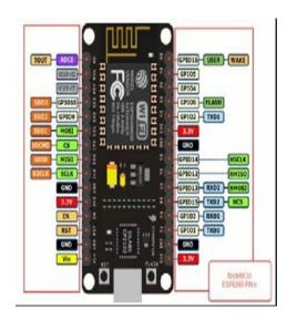
The NodeMCU ESP8266 enchancment board comes with the ESP-12E module containing ESP8266 chip having Tensilica Xtensa 32-bit LX106 RISC microprocessor. This microprocessor helps RTOS and operates at 80MHz to a hundred and sixty MHz adjustable clock frequency.
