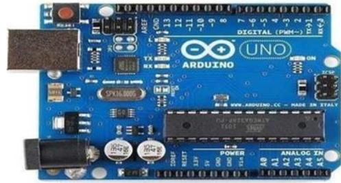
Arduino could be a micro controller, it consists of has 14 digital I/O pins and 6 analog I/O pins, a 16 MHz quartz, a USB connection, an influence jack, an ICSP header and a push button. The Uno board and version 1.0 of Arduino Software (IDE) were the reference versions of Arduino, now evolved to newer releases. The Uno board is that the first in a very series of USB Arduino boards, and therefore the reference model for the Arduino platform.
