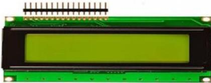
LED (Liquid Crystal Display) could be a style of flat panel display which uses liquid crystals in its primary sort of operation.
