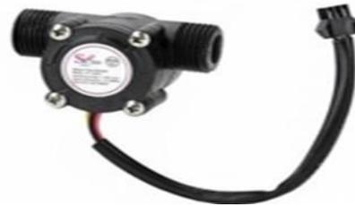
A water flow sensor may be a scientific device that's accustomed measure the flow of water. The sensor comes with three wires: red (5-24VDC power), black (ground) and yellow (Hall effect pulse output). By counting the pulses from the output of the sensor, one can easily calculate water flow. Each pulse is approximately 2.25 milli litres.
