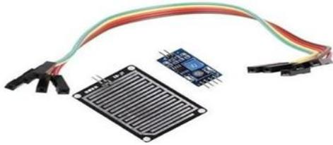
The rain sensor module is a straightforward tool for rain detection. It may be used as a switch when raindrop falls through the raining board. It may be used for measuring rainfall intensity. The module features, a rain board and a separate board for more convenience, power indicator LED and an adjustable sensitivity through a potentiometer.
