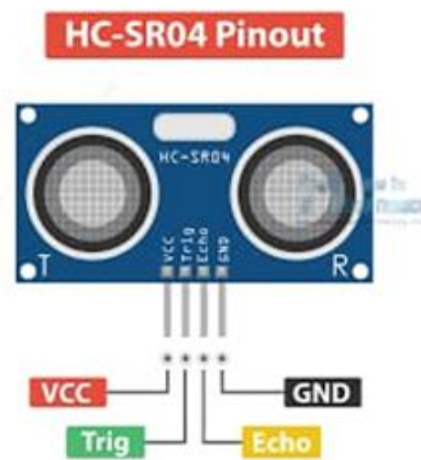
Fig.3 Ultra Sonic Sensor with pins
