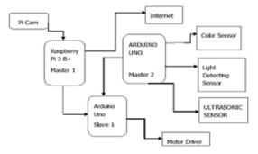
Here above represents the Block diagram implementation of CNN based self driven vehicle.
