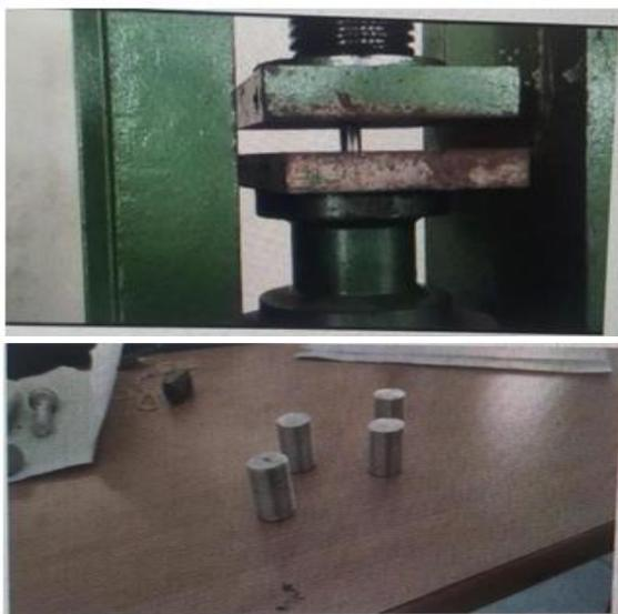
Fig 2.1 Before compression of specimen
