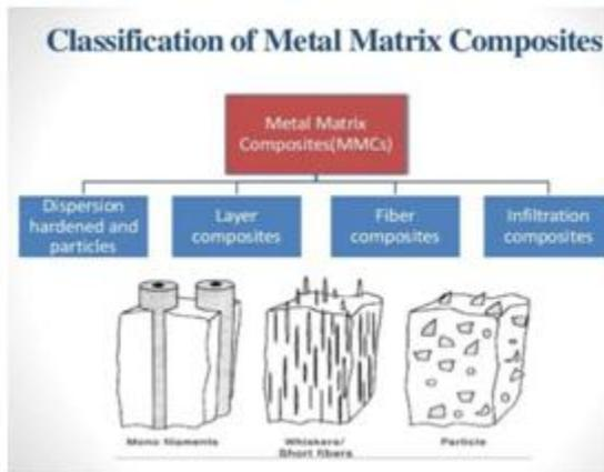
Fig 1: Classification of Metal Matrix Composites
