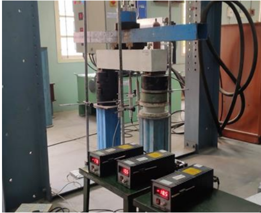
Fig 4: Experimental setup for flexural study
