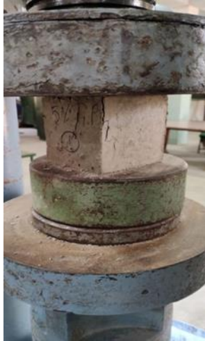
Fig 2: Experimental setup for compressive strength
