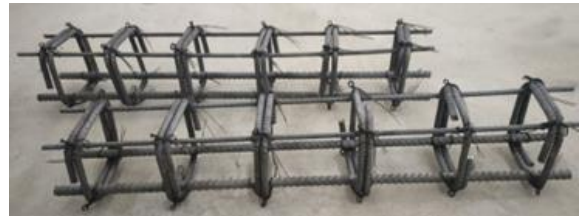
Fig 3: reinforcement details of the beam
