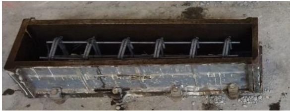
Fig 4 Reinforcement of lightweight concrete
