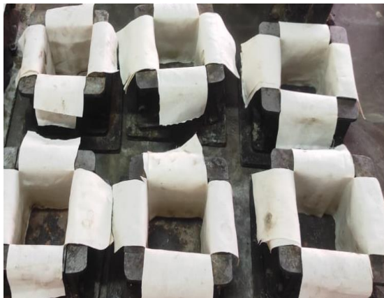
Fig 1 Mould preparation to cast cube specimens
