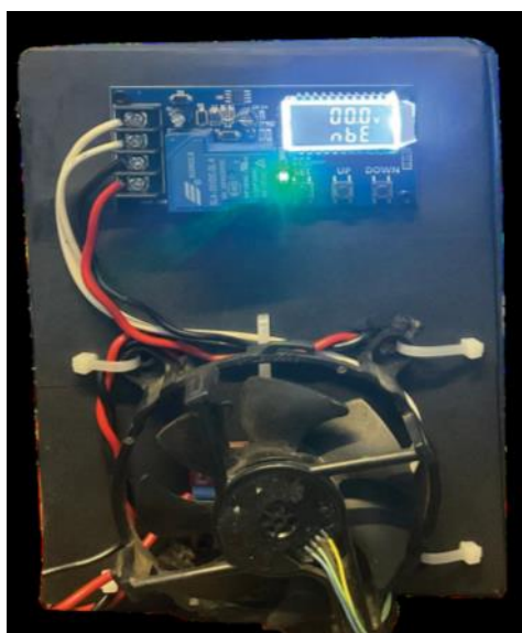
Fig 23. Charge monitoring system
