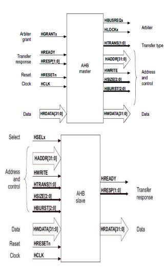
shown in Fig. 4. Here HCLK is used to get output allocated to the controller, and zero otherwise. HRESTn is used to reset the master to default conditions, BUSREQ is the bus request
