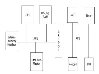
A typical AMBA Advanced High-performance Bus system designs the following components [4]:
