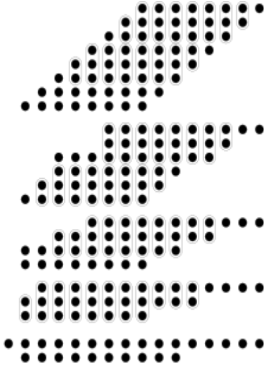
Figure 1: 16-bit Wallace tree multiplier
