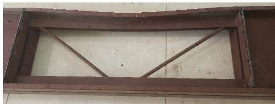
Fig.4.5 Deformed Shape of P2 specimen
