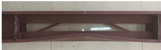
Fig.4.4 Deformed Shape of O4 specimen
