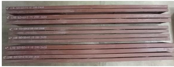
Fig.4.2 Fabricated specimens - O series
