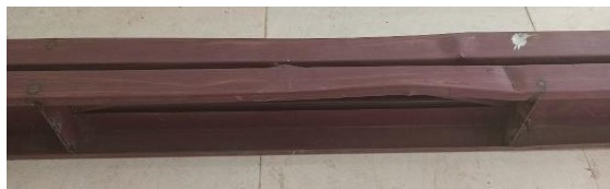
Fig.4.3 Deformed Shape of O3 specimen
