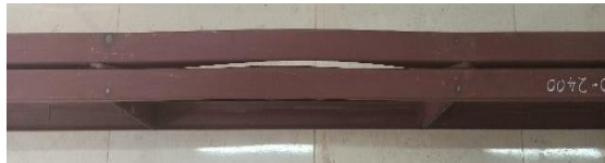
Fig.4.8 Deformed Shape of P1 specimen
