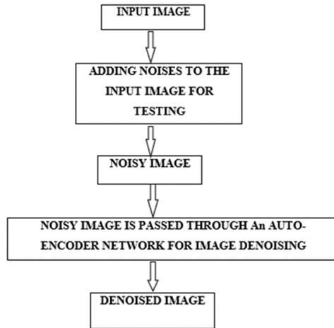
Figure 1: Flow chart of Image denoising using proposed model
