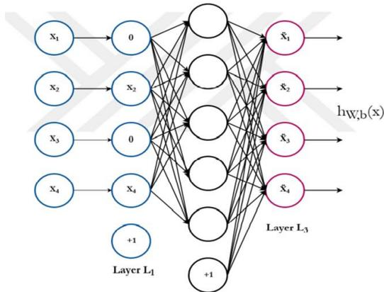
Figure 3: Example denoising auto encoder architecture
