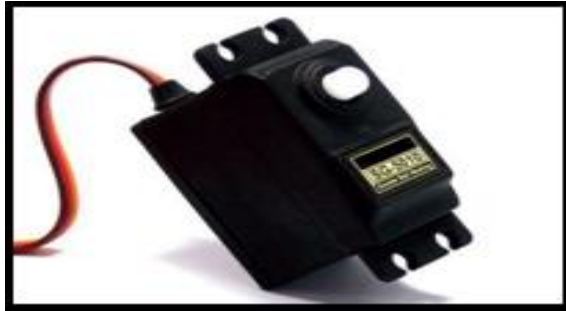
Fig.7. Servo motor (180 degree rotation)
