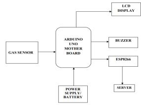
Fig. Block Diagram of Underground Drainage Monitoring System
