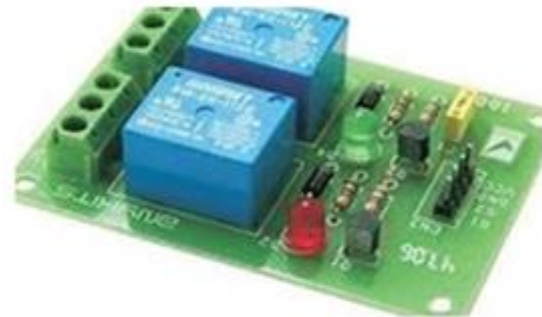
Figure 13: Relay driver circuit
