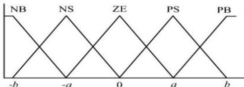
Fig. 7 Membership function for inputs and output of fuzzy logic controller.
