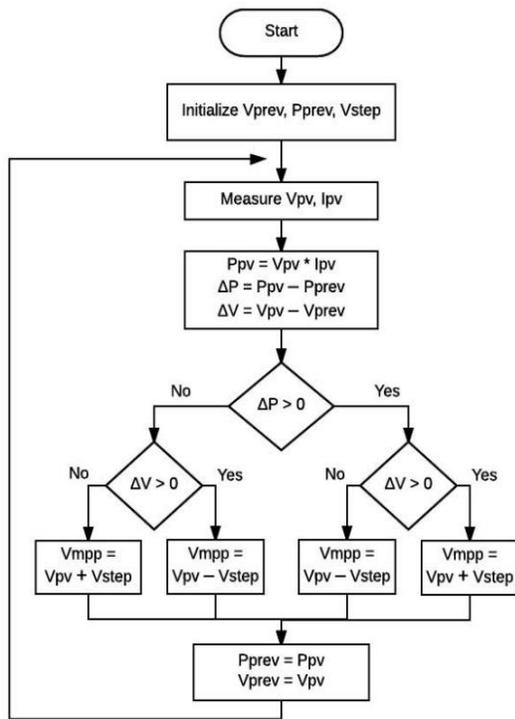
Fig. 4 Flow chart of Perturbation and Observe algorithm.
