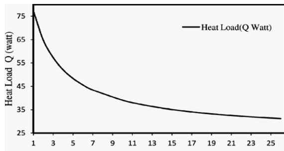
Fig. Heat Load vs. Foam Thickness
