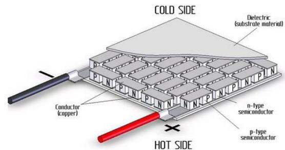
Fig: 3.1 construction diagram of PELTIER
