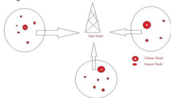
Fig 1. Sink Node in Wireless Sensor Network
