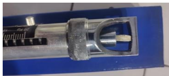
Figure 3: Hardness Testing with Monsanto Hardness Tester
