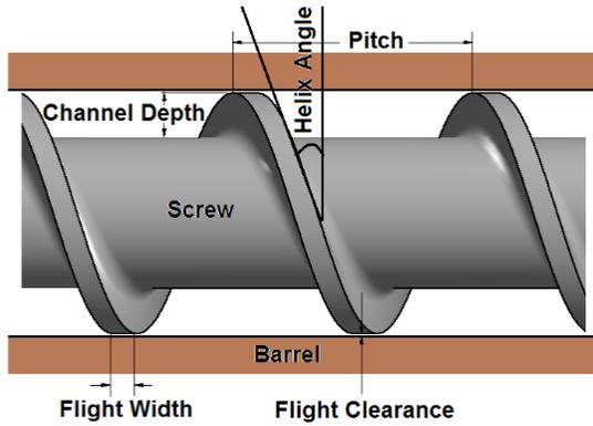
Fig. 7. Screw Diagram [5]
