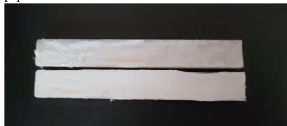
(Fig 2) Silicone strands reinforced with starch and silicon dioxide
