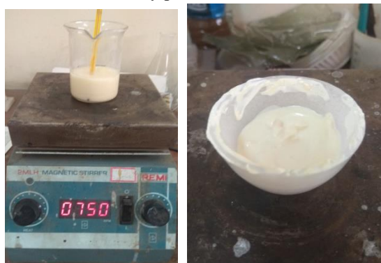
Figure 3: Y-TiO 2 solution under stirring Figure 4: Y-TiO 2 precipitate
