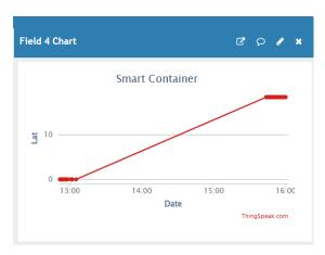
The GPS will track the actual location if the container at anytime from anywhere. It will provide us a precise location in form of latitude and longitude which can be seen from the above results.
