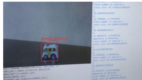
Image (3) when ambulance is present: count as vehicle1 but displays ambulance is detected.
