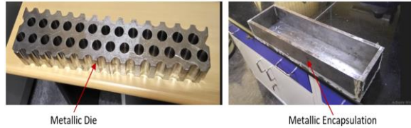
Fig. 3 Metallic Die and Metallic Encapsulation for fabrication of Ceramic Pad
