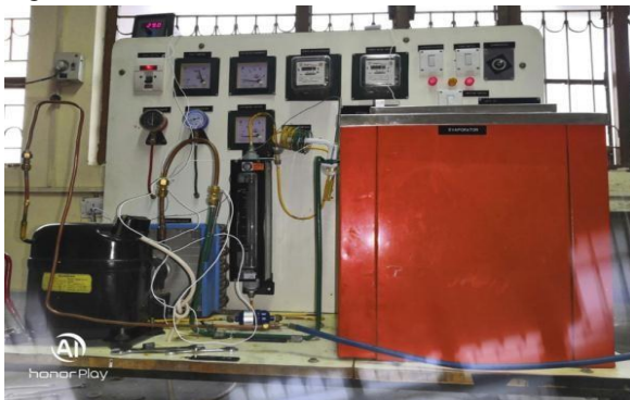
Fig.4: Shows the actual setup for vapour compression refrigeration test rig in which R438a Refrigerant is used as working fluid along with the Al nanoparticle by weight of refrigerant
