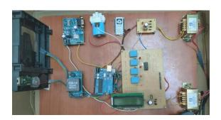
All the required components were bought, it was assembled properly then the required source code for was done in the Arduino IDE by installing allthe required libraries. Then a soldering kit was bought and with help of some professionals we soldered the whole circuit and it was temporarily pinned in a board.
