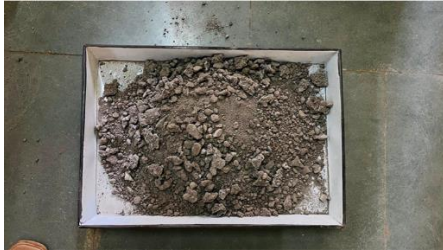
Fig. 2 BOF steel slag in aggregate form
