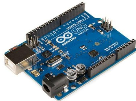
Fig1. Diagram for Arduino UNO
