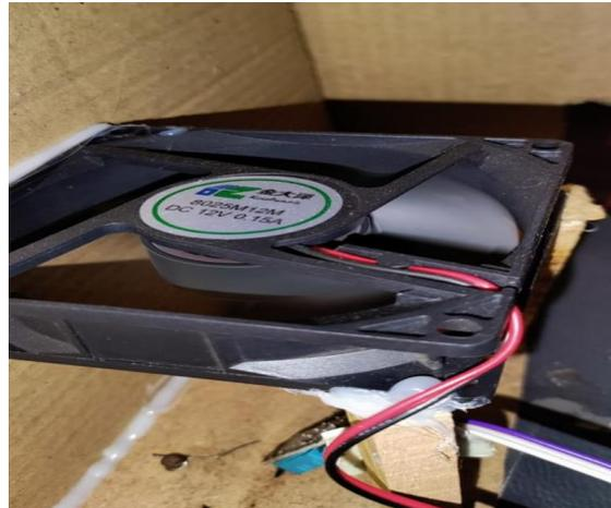
d. Fan will rotate for the temperature less than 47.5 degrees, above it will stop.
