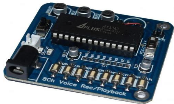
Fig6: APR33A3 Voice Playback Module
