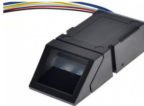
Fig5: R307 Fingerprint Module
