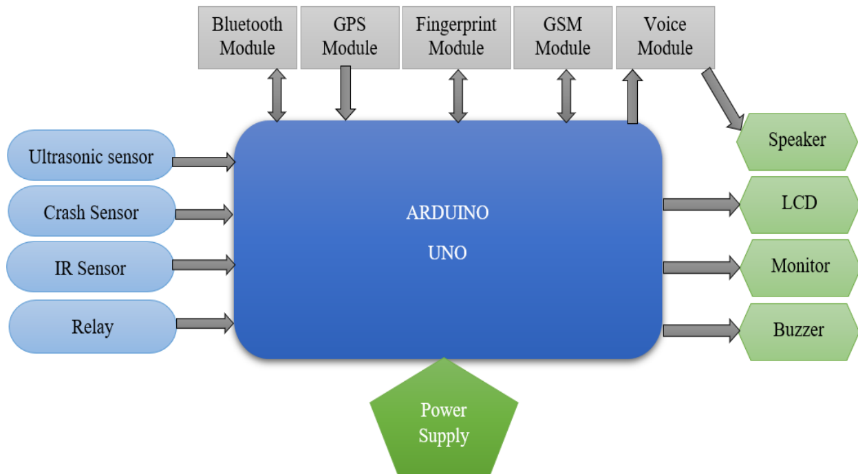
Fig.3.1. an architectural framework of smart way of motorcycle problems solved based on IoT.
