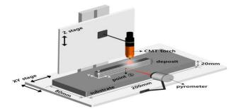
Above figure show the instrumental setup for CMT torch must have the capacity or the X and Y axis stage can be moved according to the program or machine setup so both the wire arc additive manufacturing can be possible in this method.
