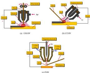
GTAW produces high quality welds using an open arc between a non-consumable tungsten electrode and workpiece. It is also referred to as TIG (Tungsten Inert Gas) welding. There is no slag or spatter, and it requires little post-weld cleaning. It is easily used in all welding positions and has been extensively used in the aerospace, aircraft, power generation, petroleum, and chemical industries.
