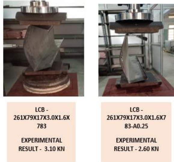
GRAPH 1. COMPARISON OF FE ANALYSIS & EXPERIMENTAL TEST RESULTS OF WEB CRIPPLING STRENGTH
