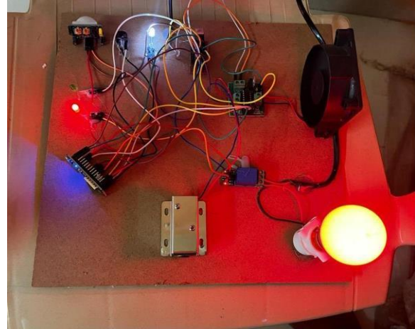
Fig2: PIR sensor sense movement red LED and buzzer turns on
