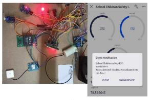
In an emergency case like an accident or smoke etc are detected. It sends notifications to register devices through the IOT server.
