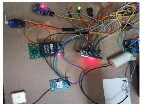
When a Valid Student ID card is swapped to the RFID Reader, Reads the card due to a valid student ID card. So Green LED is OFF"
