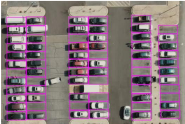
Fig 3: Segmentation of parking spaces
