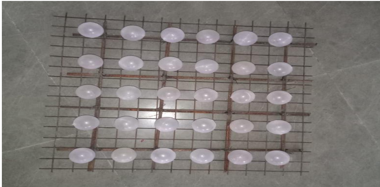
Fig. 5.3 Bubble Deck Concrete Slab.
